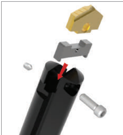
Step 1: Position the adapter into the holder.
